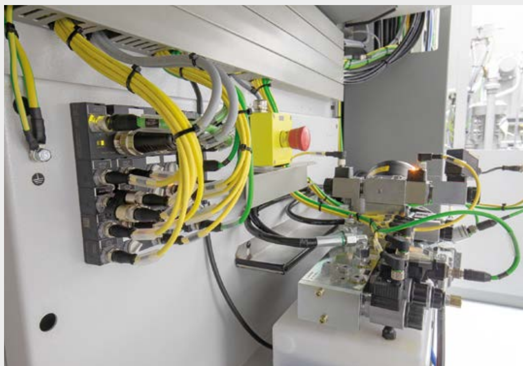
The compact Cube67 modules are installed next to the process.
